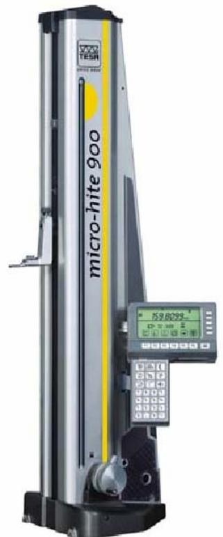
**ARG's** inspecting equipment list includes the "Micro-Hite 900" with computer interface, allowing the Quality Control Department to provide complete dimensional data inspection reports from the measured parts.
